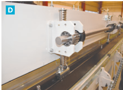
Servo-driven, heavy-duty top bar ensures minimal movement, correct press force, high capacity and is easily adjustable from the control panel.
