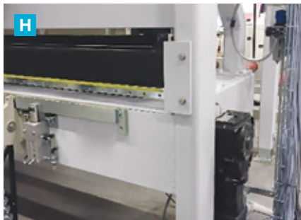
Heavy-duty pre-press and press frame to prevent deflection during operation.
