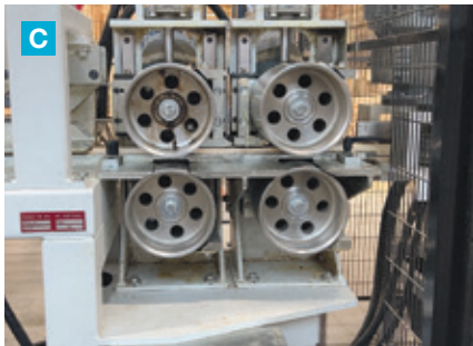
Dual set of servo-driven top and bottom motors including pneumatic brake unit. This provides fast and reliable pre-pressing of all joints.
