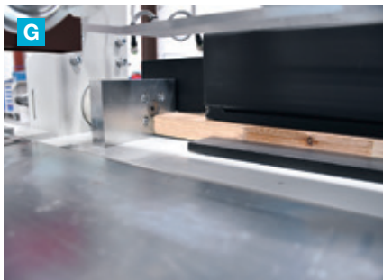
Hydraulic press station for high and correct press force. Workpieces are supported on all sides by mechanical guides to prevent movement during pressing.
