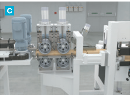
Pre-press including dual set of top and bottom motors with pneumatic brake units. This provides fast and reliable pre-pressing of all joints.
