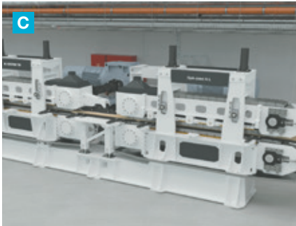
C Continuous press with continuous speed of last bottom and top caterpillar chain, torque controlled first bottom and top caterpillar chains for exact press force required per workpiece joint.
