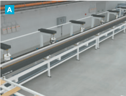
A Alignment station and continuous press, automatically adjustable in regard to the workpiece dimensions. Dimension adjustment either from operator panel or through external software interface.
