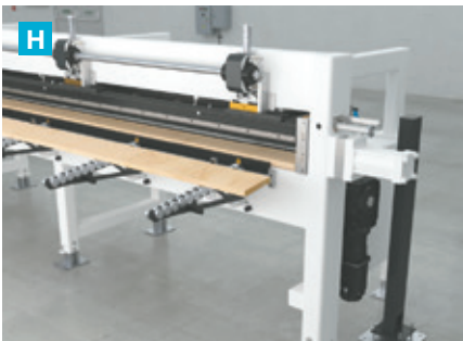
Heavy-duty press frame to prevent deflection during operation.
