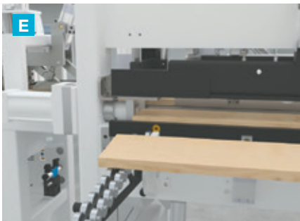
Hydraulic press station for high and correct pressing force. Workpieces are supported on all sides by mechanical guides to prevent them from moving during the pressing process.
