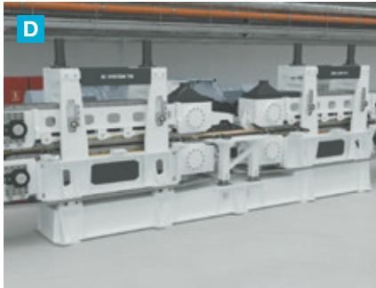
D Water cooling system for cooling the two upper caterpillar chains. Exhaust system to remove heat and provide ventilation from all four chains.
