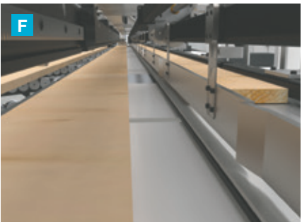
Dual channel press systems provide high capacity. While final pressing is in progress, the next workpiece is prepared for best press utilization.
