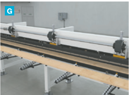
Servo-driven, heavy-duty top bar ensures minimal movement, correct pressure force, high capacity. Easy adjustment from the control panel.
