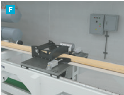
F Flying saw for continuous high-speed production, easy changeover, and high accuracy.
