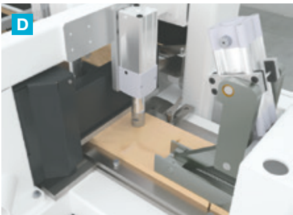
Cross-cut saw including fixed positioning of workpieces to pre-cut them to length before the press station.
