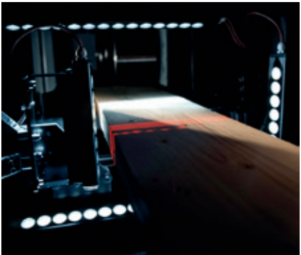
The Multi-Sensor scanning technology scans workpieces for best wood utilization.
